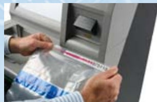
A barcode scanner is used to identify and register bags, envelopes, coupons, etc.
